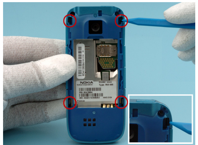
6. Release 4 clips to release the A-cover.
