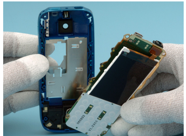
16. Remove the engine module.
