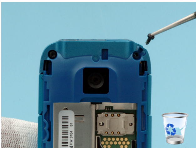
5. Use the dental tool to remove the screws.
