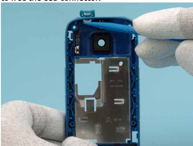
17. Remove the USB dust cap. Use the SS-93 tool and push the cap from inside the device.
