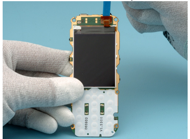
26. Use the dental tool to lift microphone.
