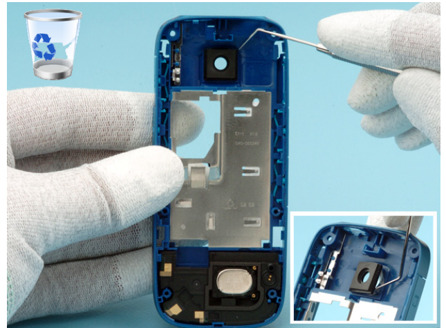
20. Remove the camera gasket as one piece.
