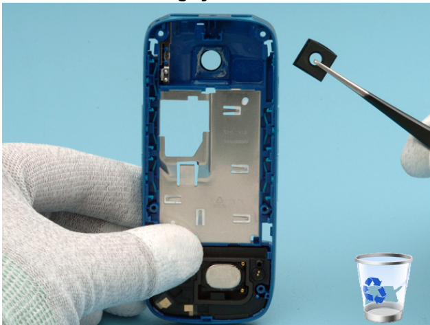
19. Remove the charge jack with tweezers.
