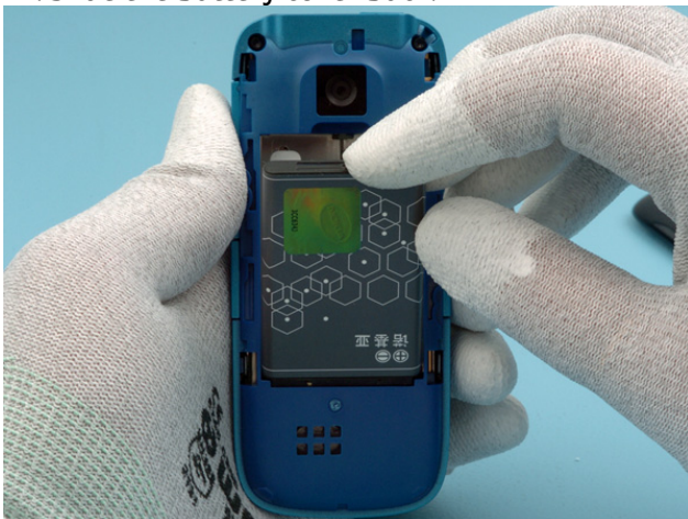
3. Lift and remove the battery.
