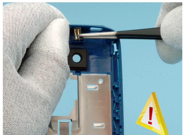
18. Carefully bend the C-cover slightly backwards with your thumb and lift the back side of the charge jack with tweezers.
