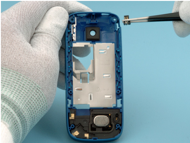
19. Remove the charge jack with tweezers.
